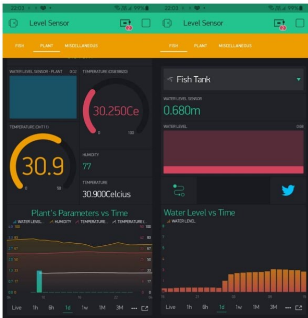
Figure 10 Blynk Dashboards displaying sensor data for Fish Tanks and Plant tray
