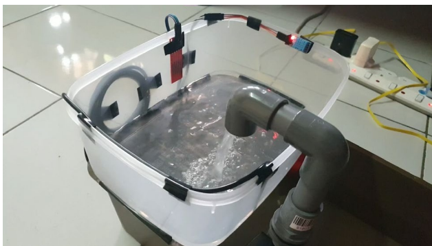
Figure 9 Water is pumped when water level readings exceed 8 liters at Fish Tank
