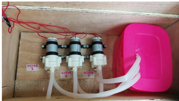
Figure 12: Actual project hardware connection and construction (Motor/Water Pumps and water tank).
