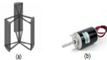
Figure 6: VAWT Configurations: (a) Wind Turbine with 3 Blades Design, (b) DC Motor
