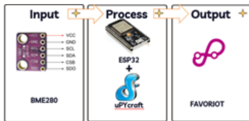
Fig 2. The block diagram of Emergency Staircase Monitoring System
