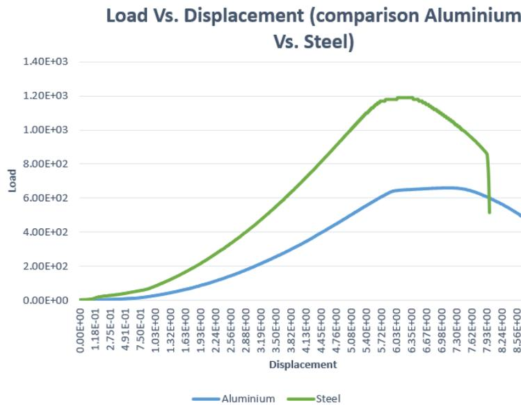
Figure 2: Load vs Displacement for aluminium and steel
